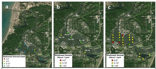
**Figure 3**: Locations of sediment sampling sites with detected PCBs. Panel a shows all 2019 sampling stations where PCBs were detected, colored by the shallowed depth of detection; Panels b and c show the 2019 and 2000 sampling stations, respectively, where at least one sample had PCB concentrations exceeding the 1 ppm regulatory limit. Marker color indicates the shallowest depth in which a sample exceeded the limit.
