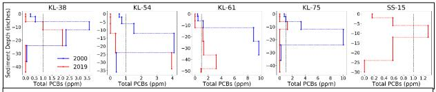
*Figure 4*: PCB contamination profiles for the sampling sites where PCB samples from 2019 exceeded the regulatory limit of 1 ppm: KL-38, KL-54, KL-61, KL-75, and SS-15. Profiles from 2019 are shown in red, and where possible, profiles from 2000 are in blue.
