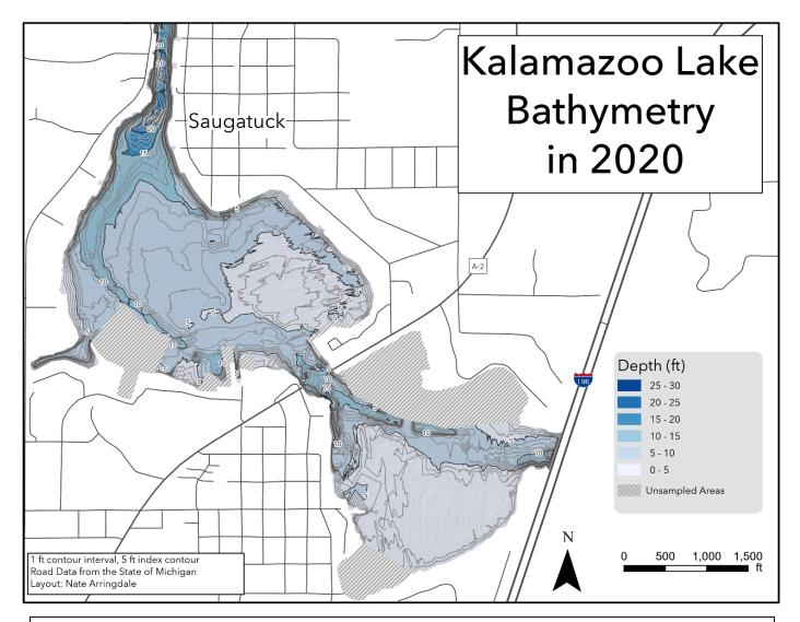
*Figure 5:* Updated bathymetric map for Kalamazoo Lake and the Kalamazoo River channel near Saugatuck and Douglas, MI. 1 ft contours are displayed, with bold lines at each 5 ft interval. Areas marked with slashed lines were not sampled due to dock presence or persistent EWM presence.
